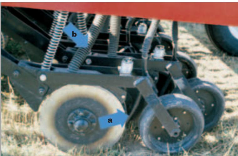
To plant companion crops 1 to 2 inches deeper than alfalfa in a single pass, place the drop tube for alfalfa behind coulters but before the packer wheel (a) and place the drop tube for the cover crop between coulters (b).
