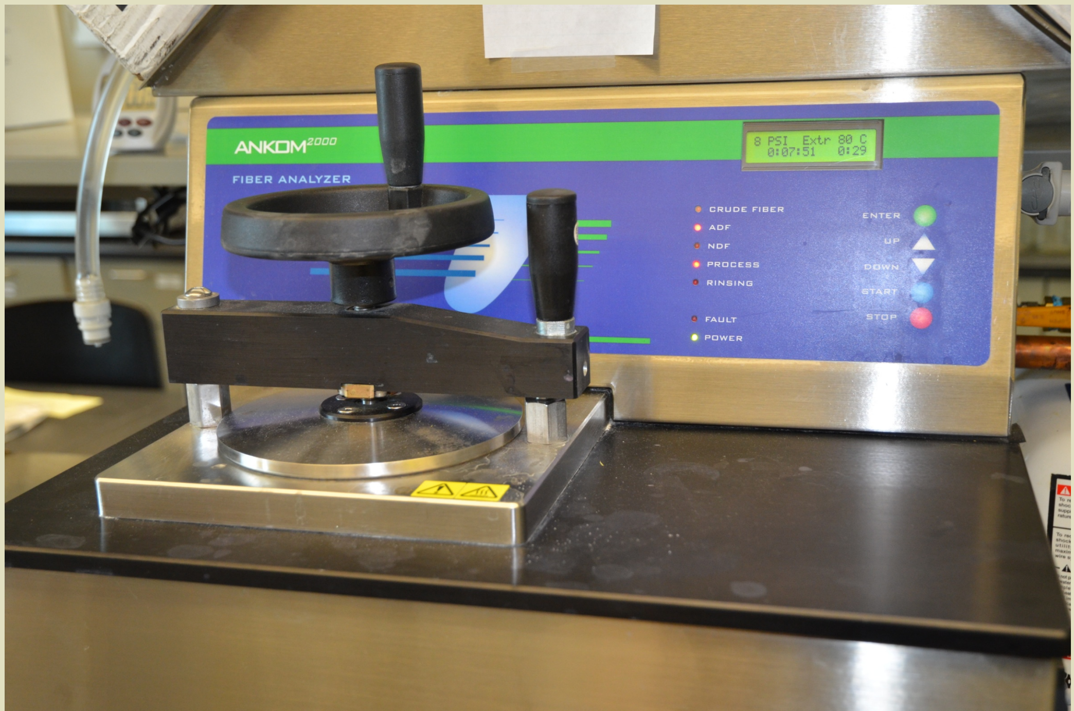
Figure 4. Ankom 2000 Fiber analyzer used to measure ADF.
